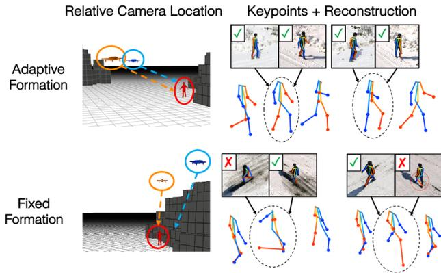
Fig. 10: Reconstruction comparison with and without adaptive formation planning. The formation planning keeps camera at a low tilt angle and significantly improves reconstruction. Without formation planning, the UAVs goes upward to avoid mound. The skeletal keypoint detection fails often for footage collected with fixed formation, resulting in poor reconstruction.
