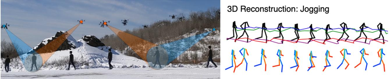
Fig. 1: We present a multi-UAV system for 3D human reconstruction in the wild. Our framework coordinates the motion of multiple aerial cameras to optimally reconstruct the dynamic target’s 3D body pose while avoiding obstacles and occlusions. We deploy the system in challenging real-world conditions and target motions such as jogging and playing soccer.
