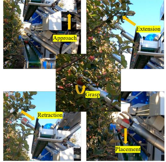
Fig. 3. Five sequential actions of robotic arms in harvesting operation.
