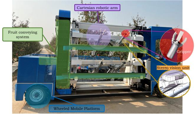
Fig. 1. The multi-arm apple harvesting robot presented in this work.
