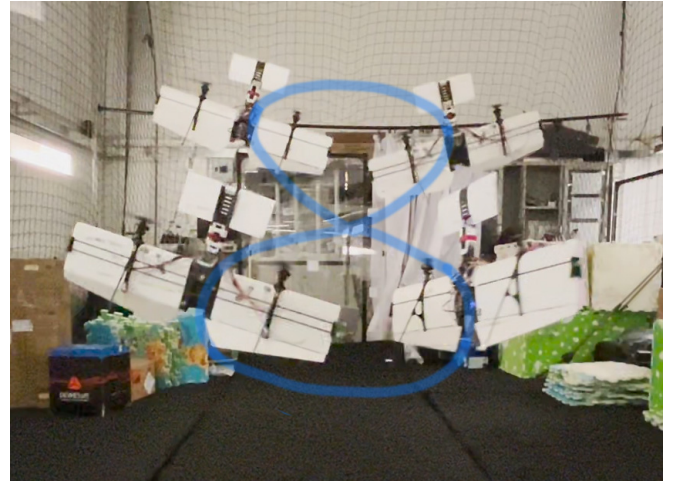
Fig. 7. The overlaid snapshots of Hong He when it tracks a 3D figure-of-eight trajectory with continuous yaw rotation.
