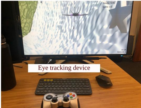
Fig. 2: The experimental setup with the eye tracking devices to get the attention profile of the pilot
