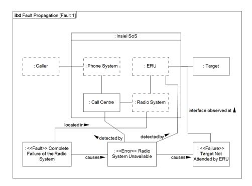
Figure 19: Fault Propagation View for Fault 1
