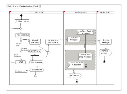
Figure 24: Fault Activation View (initiate rescue process) for Fault 1
