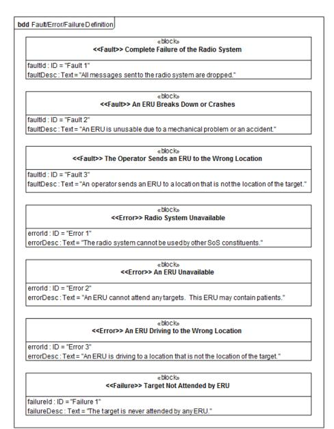
Figure 18: Fault/Error/Failure Definition View
