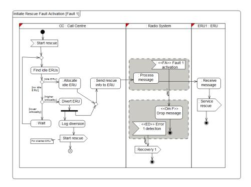
Figure 4: Fault Activation View (initiate rescue process) for Fault 1
