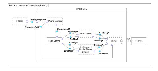
Figure 3: Fault Tolerance Connections View for Fault 1
