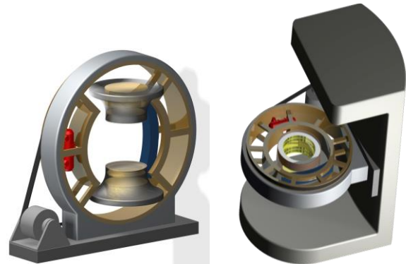
Fig. 4. Rotating CT/MRI. (Left) Compact low field MRI with permanent magnets with a rotating gantry located perpendicularly. (Right) Design for vertical imaging
