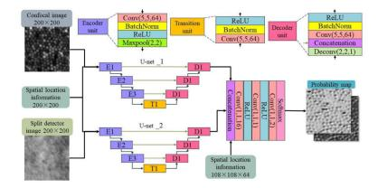
**Figure 2.** Diagram of the CNN architecture used in the proposed method.
