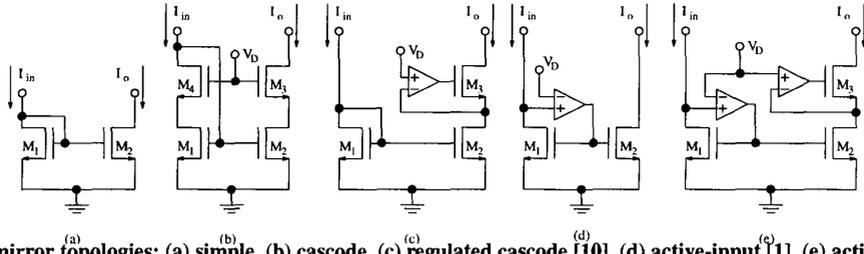
Fig. 5: Current mirror topologies: (a) simple, (b) cascode, (c) regulated cascode [10], (d) active-input [1], (e) active-input regulated cascode [12]
