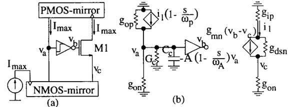
Fig. 4: Steady state representation of WTA current-mode circuit. (a) Circuit diagram, (b) small signal equivalent circuit
