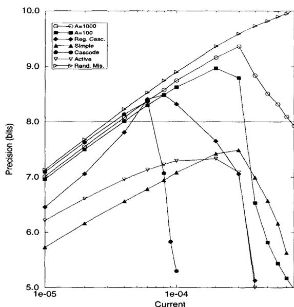
Fig. 6: Resolution (in bits) as a function of working current for different current mirror topologies: simple, cascode, regulated cascode, active-input, and active-input regulated-cascode with voltage gains  $A=100$  and  $A=1000$
