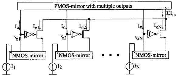
Fig. 2: Circuit diagram of complete current-mode WTA
