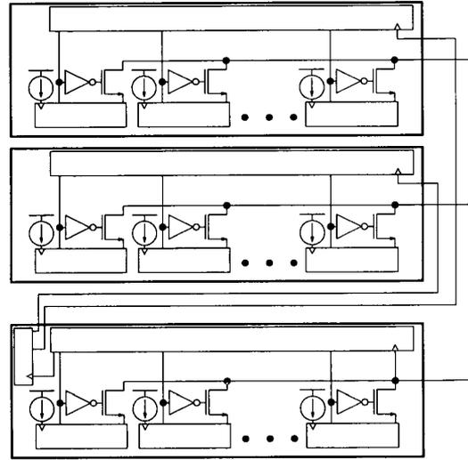
Fig. 3: Modular inter-chip connection for current-mode WTA
