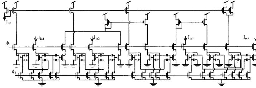
Figure 6: Root mean square (vector sum) normalization circuit
