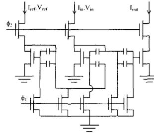
Figure 5: Dynamically restored squaring circuit
