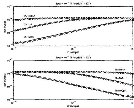
Figure 10: RMS normalization circuit results
