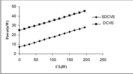
Figure 3. Power dissipation of DCVS and SDCVS level shifters for various  $C_L$ .
