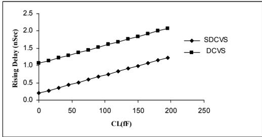
Figure 4. Delay of DCVS and SDCVS level shifters for various  $C_L$ .
