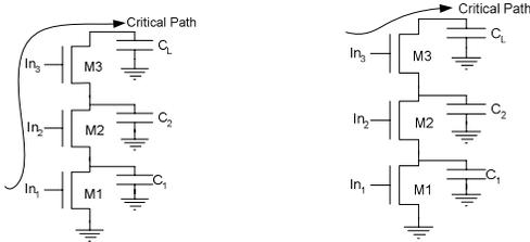
Figure 5. Transistor ordering
