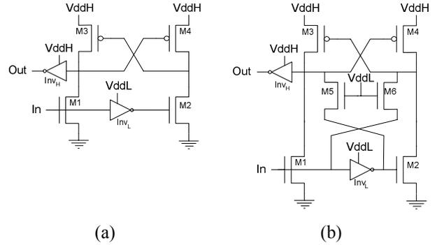
Figure 2. (a) The DCVS level shifter (b) The SDCVS level shifter [12].
