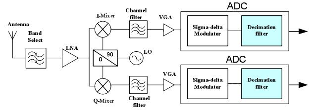
Figure 2. Direct conversion homodyne receiver architecture
