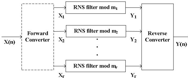
Figure 1. RNS based FIR filter
