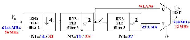
Figure 3. Programmable decimation filter for WCDMA/WiMAX
