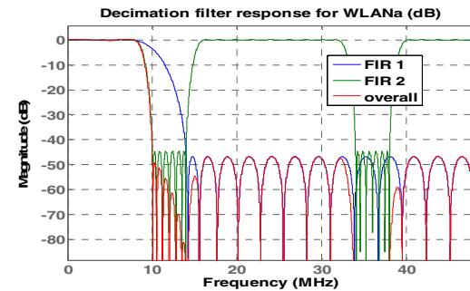
Figure 6. Decimation filter response for WLAna
