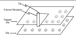
Fig. 6: Two identical array coil surfaces can be packaged to face one another to generate a motoring action between the two surfaces. This action will control the vertical motion as well as rotational motion along any chosen axis between any coils. This provides the tip with "approach" motion as well as with lateral motion over a region for the single tip.
