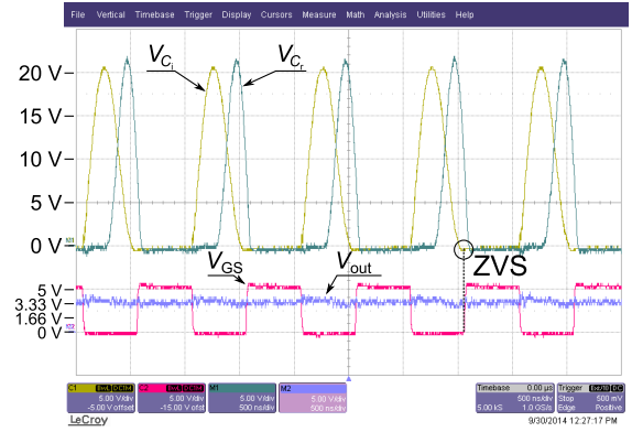
Fig. 6. Measured waveforms for the implemented class-E converter.
