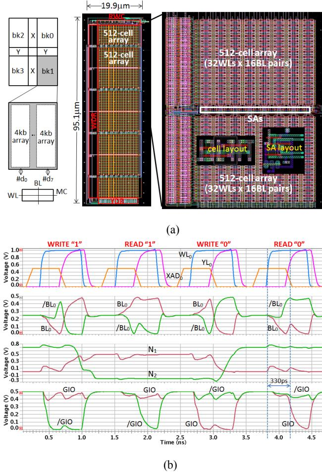
Fig. 6 (a) Layout and (b) simulated waveforms of 4-kb array in 128-kb SRAM core with 4 banks (bk0-bk3).
