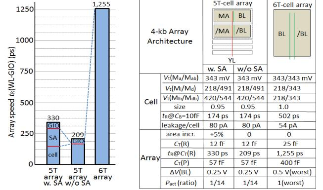
Fig. 7 (a) Expected speed improvement and (b) comparisons with a counterpart 6-T cell array.  $V_{DD} = 0.5 \text{ V}$ ,  $V_{WL} = 1.0 \text{ V}$ ,  $V_{DH} = 0.7 \text{ V}$ , and  $V_{SL} = 0.2 \text{ V}$ .  $t_R$ ; WL-GIO delay.  $\Delta V(BL)$ ; voltage swing on BLs.
