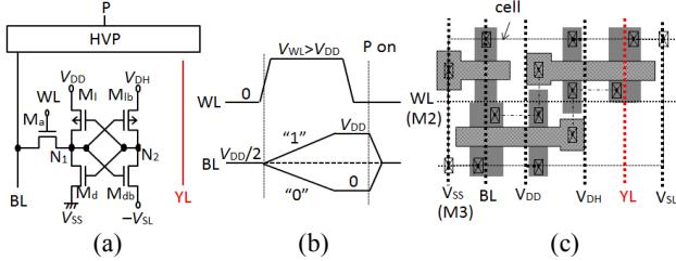
Fig. 1 Concept of proposed 5T cell. (a) Circuit, (b) timing, and (c) layout. P: precharge pulse.
