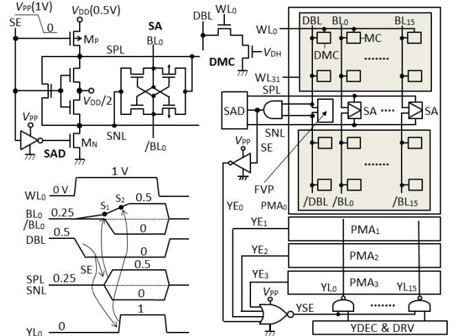
Fig. 5 Peripheral circuits and timing diagram of the array.
