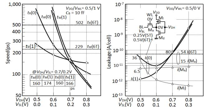
Fig. 2 Speeds and leakage current vs.  $V_{DH}$  and  $V_{SL}$ .
