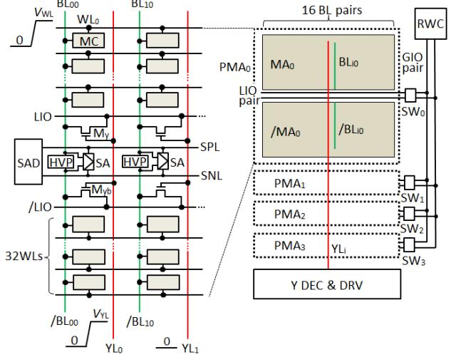
Fig. 4 Concept of the proposed open-BL 5T-cell array.
