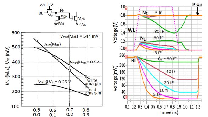
Fig. 3 (a) DC characteristics of 5T cell and (b) waveforms at  $V_{DH}/V_{SL} = 0.8/0.3$  V.
