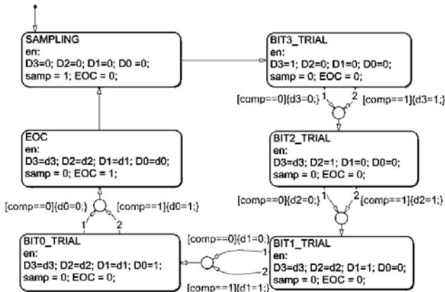
Fig. 2. State transition diagram of a 4-bit SAR-digital.
