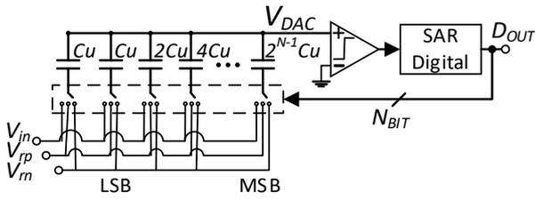
Fig. 1. SAR ADC Schematic.
