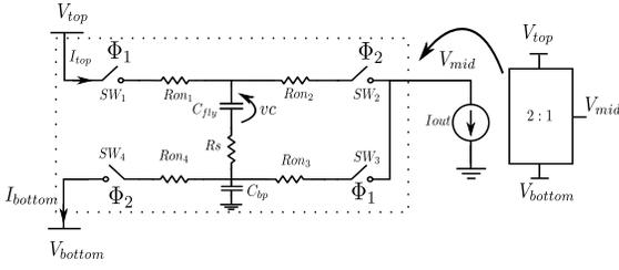
Fig. 2. Circuit representation of a 2 : 1 SC converter
