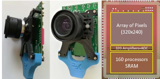
Fig. 1. The demo (left and middle); vision Chip microphotograph (right).
