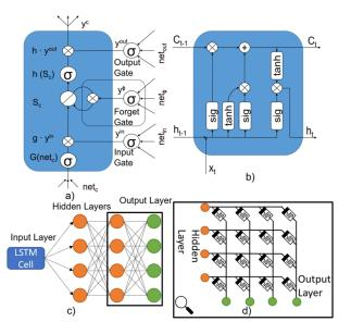
Fig. 1. a) LSTM cell with forget gate, b) Modern representation of an LSTM cell [17], c) Network used for predicting and classifying faults in wind turbines blade, d) Memristor crossbar array used for the neurons in an ANN
