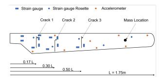
Fig. 2. Sensor Layout on wind turbine blade
