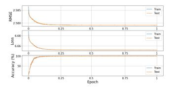
Fig. 3. Classifier's training results, showing that the classifier was accurate after less than one Epoch
