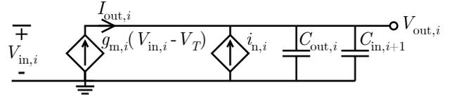
Fig. 3. Circuit model of the  $i^{\text{th}}$  inverter in a chain.
