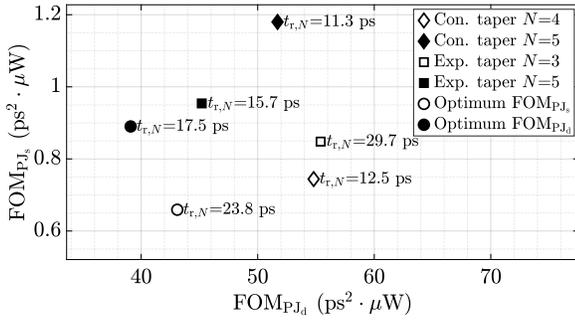
Fig. 5. Circuit simulations with  $\Gamma = 100$  in 22nm FD-SOI that verify the numerical simulation results.
