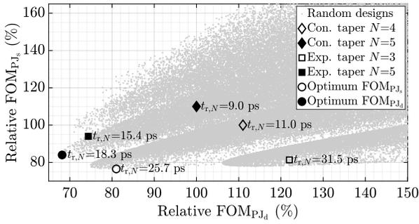
Fig. 4. Numerical simulations of the  $FOM_{PJ_s}$  and  $FOM_{PJ_d}$  design space including the randomly generated designs with  $\Gamma = 100$ , showing that the simple exponential tapers are near-optimal for these individual metrics. The axes are relative to the constant taper designs. A lower FOM is better.
