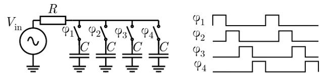
Fig. 1. Clock signals driving the switches in a 4-path filter.
