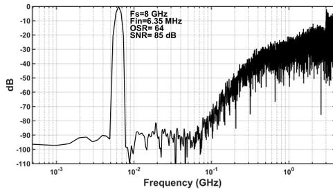
Fig. 8: Output Power Spectral Density for lowpass ADC
