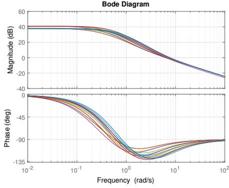
Fig. 2: Bode plot of the generated 2 stage opamp specifications
