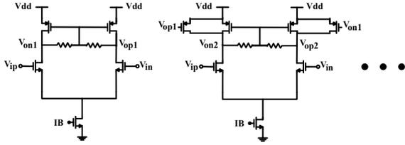
Fig. 7: Schematic of 4 stages opamp
