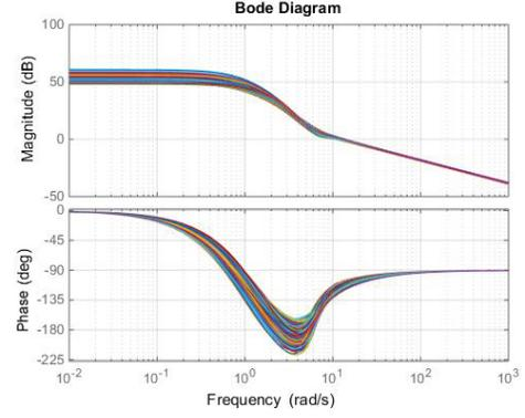
Fig. 5: Bode plot of the generated 4 stages opamp specifications
