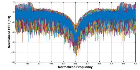
Fig. 6: PSD of 4th order bandpass  $\Sigma\Delta$  ADC using 4 stages opamp
