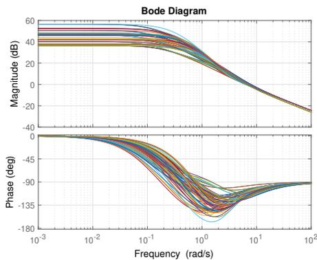
Fig. 4: Bode plot of the generated 3 stages opamp specifications
