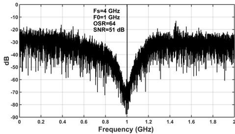
Fig. 9: Output Power Spectral Density for bandpass ADC
