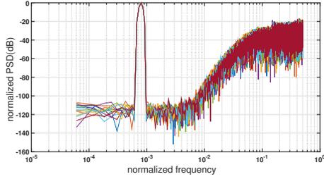
Fig. 3: PSD of 4th order lowpass  $\Sigma\Delta$  ADC using 2 stage opamp
