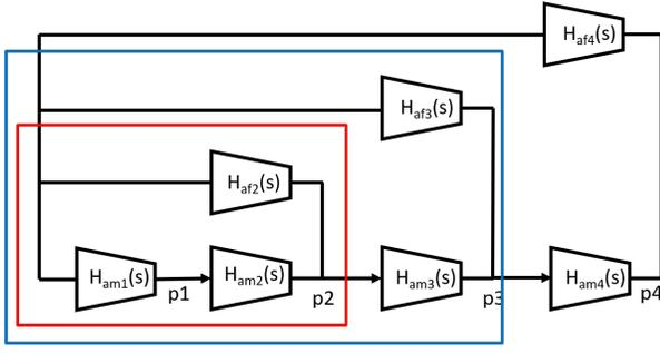
Fig. 1: Multistage Feedforward Compensated Opamp
