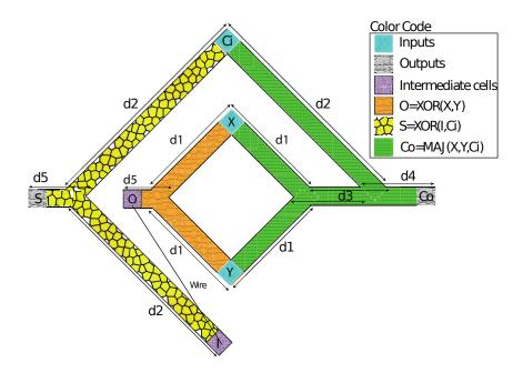
FIG. 1. Spin Wave Based Full Adder.
