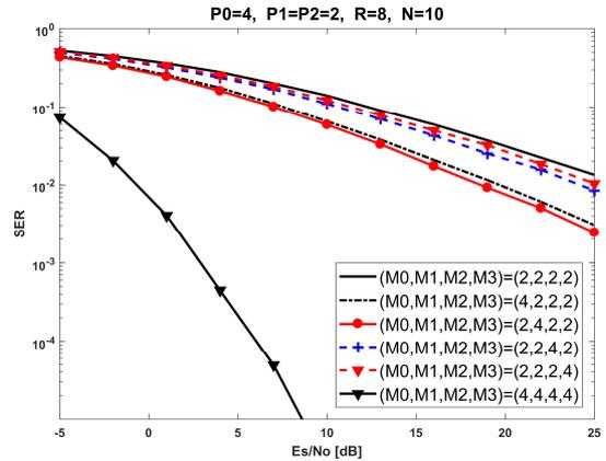
Fig. 4. ZF receiver performance for different numbers of antennas.
