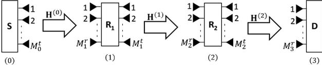
Fig. 1. Three-hop MIMO relay system.
