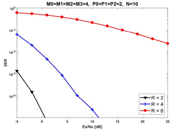
Fig. 2. ZF receiver performance for different numbers of data stream.
