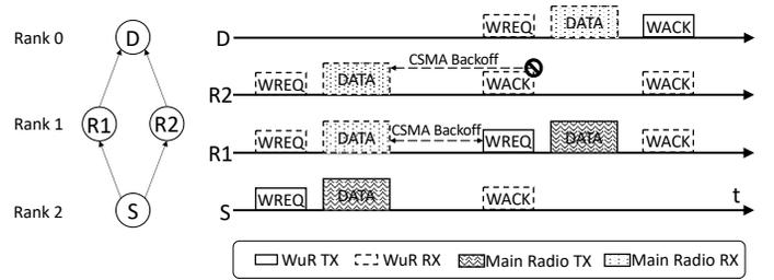
Fig. 1: Example of the algorithm in a timeline
