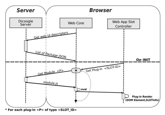
Figure 2: Dicoogle Web Core sequence diagram
