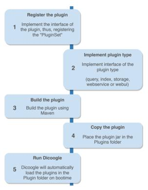
Figure 3: Workflow of the development of a Dicoogle Plugin
