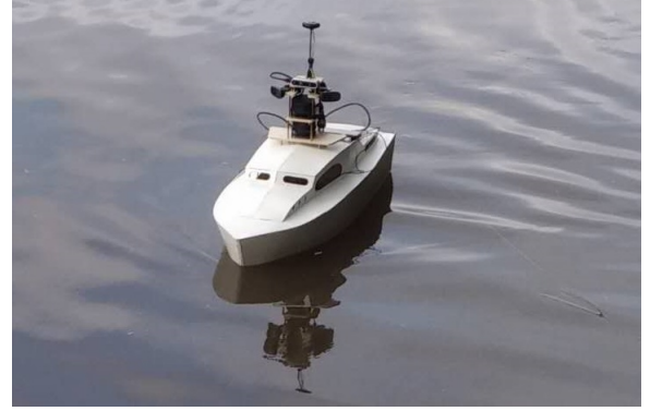
Fig. 1. Prototype vessel TIERS1 used as sensing platform for testing.
