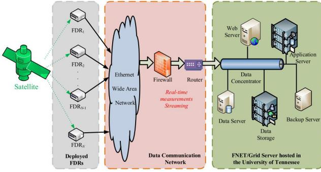
Figure 1. FNET/GridEye achitecture.
