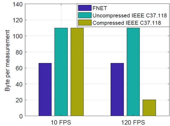
Figure 5. Data packet compression.
