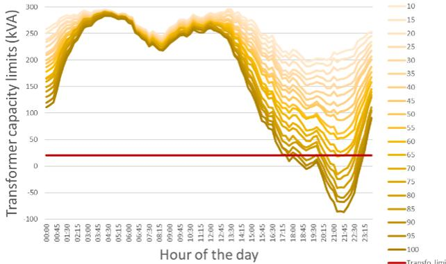
Figure 5: Average transformer capacity available for each EV penetration rate, without controlled charging
