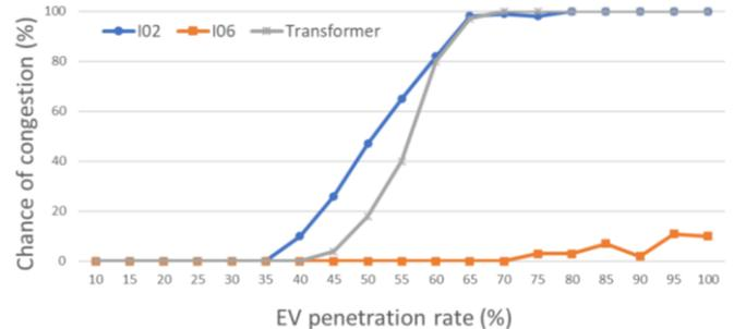
Figure 3: Congestion occurrence in feeders I02, I06 and transformer for each EV penetration rate
