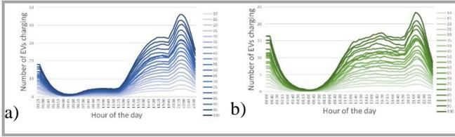
Figure 4: Simultaneity of uncontrolled charging for each penetration rate. a) during weekdays, b) during the weekend
