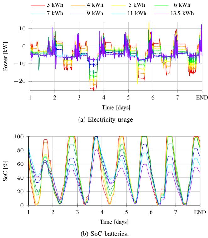
Fig. 4. Electricity usage and battery SoC in week A for varied battery sizes
