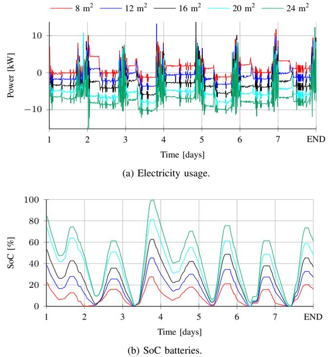
Fig. 3. Electricity usage and battery SoC in week A for varied PV areas
