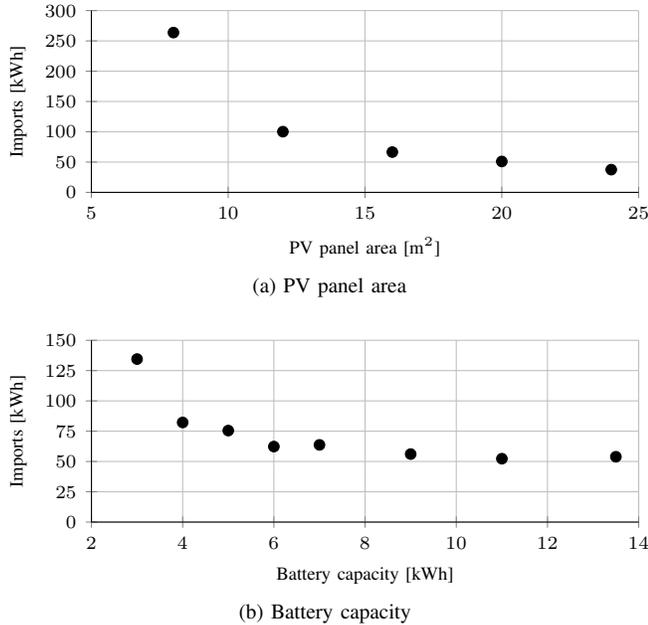
Fig. 5. Necessary electricity imports for the considered battery capacities and PV panel areas during week A.
