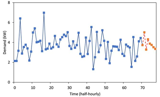
Fig. 5. Baseline estimation showing input data and output of the LSTM model.
