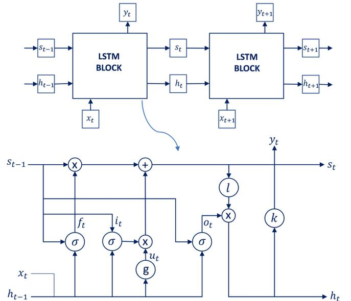
Fig. 2. LSTM RNN architecture.
