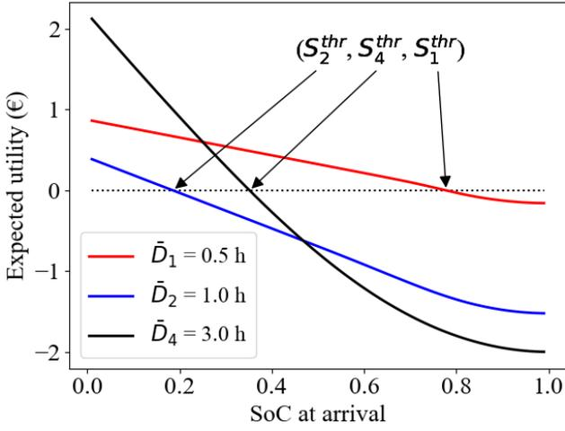
Fig. 2: Expected utility, defined in (3), for different classes, for a pricing policy  $a = 3\text{€}$  and  $d_{thr}=45\text{min}$ . EV users of class 1 (resp. 2 and 4) decide to charge if their SoC at arrival is lower than 78% (resp. 20% and 37%). Given that the parking duration has a positive impact on energy received but a negative one regarding the probability to pay the parking fee, the relation between  $S_i^{thr}$  and  $\bar{D}_i$  is not trivial, here not monotonic.
