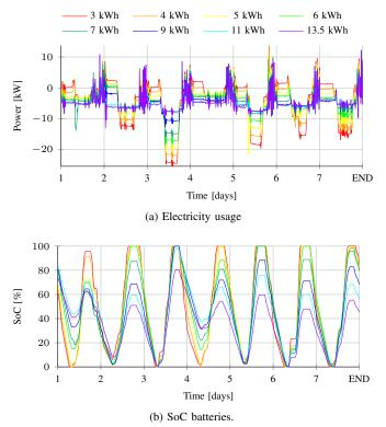
Fig. 4. Electricity usage and battery SoC in week A for varied battery sizes
