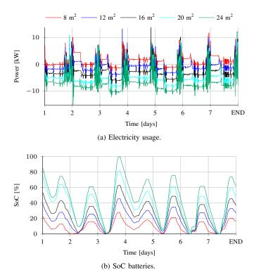
Fig. 3. Electricity usage and battery SoC in week A for varied PV areas
