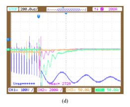
Fig. 7. Experimental short circuit tests. (a) Fault in zero-crossing range (CH1:  $v_{ou}$ , CH2:  $i_{ou}$ , CH3:  $i_T$ , CH4:  $i_B$ ). (b) Fault at a low voltage (CH1:  $v_{in}$ , CH2:  $i_{ou}$ , CH3:  $i_T$ , CH4:  $i_B$ ). (c) Fault at a high positive voltage (CH1:  $v_r$ , CH2:  $i_{ou}$ , CH3:  $i_T$ , CH4:  $i_B$ ). (d) Fault at a high negative voltage (CH1:  $v_r$  voltage across the top leg, CH2:  $i_{ou}$ , CH3:  $i_T$ , CH4:  $i_B$ ).
