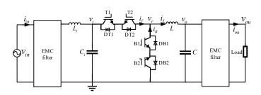
Fig. 3. Circuit diagram of the system based on the PWM ac-ac buck converter.
