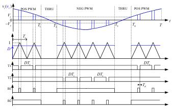
Fig. 2. PWM control of ac-ac buck converter.
