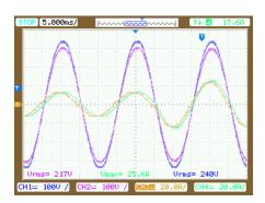
Fig. 4. Voltage regulation in experiment with a step change in load (CH1:  $v_{in}$ , CH2:  $v_{ou}$ , CH3:  $i_{in}$ , CH4:  $i_{ou}$ ).
