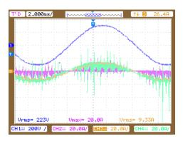
Fig. 6. Voltage regulation in experiment (CH1:  $v_{ou}$ , CH2:  $i_{\beta}$ , CH3:  $i_{ou}$ , CH4:  $i_{T}$ ).
