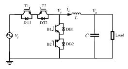
Fig. 1. Single-phase PWM ac-ac buck converter.
