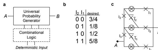
Fig. 6. **Realizing a Probabilistic Truth Table.** As an example, we will synthesize a UPG and combinational logic block which satisfies a given mapping between deterministic inputs and probabilities. (a) Combinational logic allows arbitrary mappings to be achieved. (b) The desired truth table, mapping two input bits to probabilities. (c) A UPG construction which can realize any 3-bit binary fraction.
