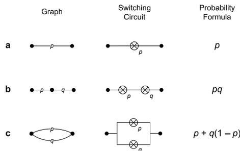
Fig. 1. **Series and Parallel Constructions.** The relationship between a graph and switching circuit is shown. There are only two ways to combine two single-pswitch circuits, both shown here. (a) Any circuit can be represented as a single pswitch. (b) Series. Only when both switches are closed is a series circuit closed. (c) Parallel. Only when both switches are open is a parallel circuit open.
