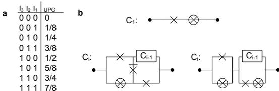
Fig. 5. **A Universal Probability Generator.** Here, we show the construction of a circuit which maps deterministic inputs to probabilities. (a) The mappings for a UPG with three deterministic input bits. (b)  $C_1$  is two switches in series. Each recursive circuit stage requires an additional four switches. Note that a single pswitch added at each stage is minimal.
