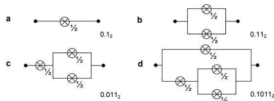
Fig. 2. **Realizing**  $F = \frac{11}{16} = 0.1011_2$ . Progressing from the least-significant to the most-significant bit in the binary representation of  $F$ , a pswitch is added in series if '0' and in parallel if '1'. The probability that each circuit is closed as a binary fraction is printed beneath the circuit. The final circuit is optimal in the number of pswitches.
