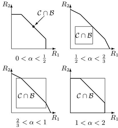
Fig. 3. Examples of  $\mathcal{C}_{\text{NE}} = \mathcal{C} \cap \mathcal{B}$  for a symmetric interference channel with normalized cross gain  $\alpha$ .
