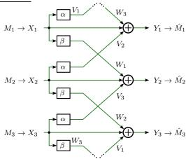
**Fig. 1.** Cyclically symmetric deterministic interference channel, K = 3.
