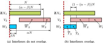
Components of received signal  $Y_1$  for the converse proof. The components are shown sideways, with the bottom pipe on the left. The dotted vertical line symbolizes the "noise level", i.e., the lower end of the vector where further down-shifts cause loss of information. The received signal  $Y_1$ is the modulo-2 sum of the three components.
