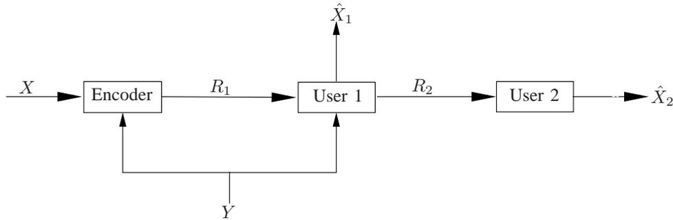
Fig. 1. A cascade rate distortion problem with three nodes (encoder, User 1, User 2), where the first two nodes have side information  $Y$ . User 1 and User 2 need to reconstruct the source  $X$ , within distortion criteria.
