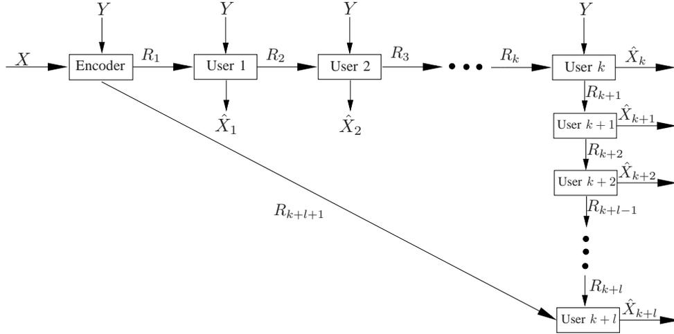
Fig. 6. A triangular rate distortion problem with  $k + l$  users, where the side information  $Y$  is known to the encoder and to Users  $1, 2, \dots, k$ , but not to Users  $k + 1, k + 2, \dots, k + l$ .
