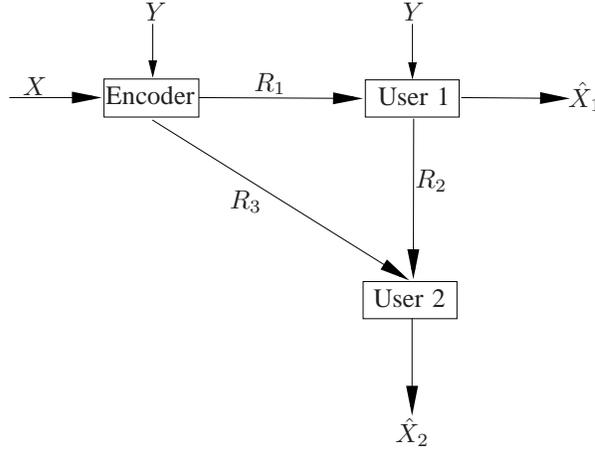
Fig. 5. A triangular rate distortion problem with three nodes (encoder, User 1, User 2), where side information  $Y$  is known to the encoder and User 1, but not to User 2. User 1 and User 2 need to reconstruct the source  $X$  to within distortion criteria.
