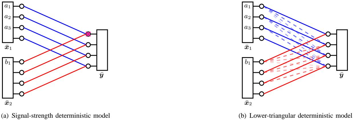
Fig. 5. Illustration of a signaling scheme that succeeds for the lower-triangular model (assuming the subspace condition (7) holds), but fails for the signal-strength model.
