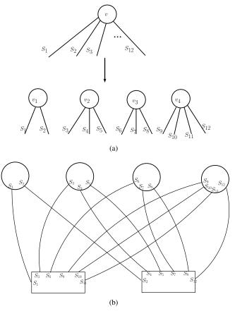
Fig. 2. Illustration of (a) variable node splitting, and (b) protograph for III-C.
