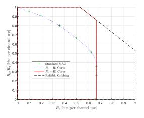
Fig. 6. The capacity region in Example 3, compared to the capacity region of the standard MAC without cribbing, and the capacity region in case of reliable cribbing, for q = 0.1. Each value of  $R_1$  is associated with two rates  $R_2$  and  $R_2''$ .
