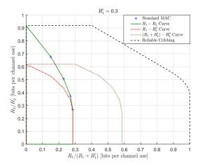
Fig. 7. The achievable region in Example 4 (see (54)), for  $p_1 = 0.01$ ,  $p_2 = 0.4$ , and  $R'_1 = 0.3$ , compared to the capacity region of the standard MAC without cribbing, and reliable cribbing. Each value of  $R_1$  is associated with two rates  $R_2$  and  $R_2''$  on the  $(R_1, R_2)$  and  $(R_1, R_2'')$  curves.
