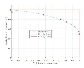
Fig. 5. The capacity region of Example 2 ((45a)-(45c)), compared to the capacity region of the standard MAC without cribbing. Each value of  $R_1$  is associated with two rates  $R_2$  and  $R_2''$ . The capacity region in case of reliable cribbing coincides with the  $(R_1, R_2'')$  curve.
