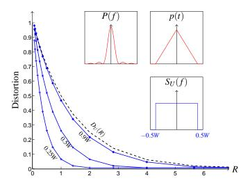
Fig. 6: The DRF of the PAM signal (16) for three values of sampling rate  $1/T_0$  compared to the Nyquist rate W of  $U(\cdot)$ . The DRF of the baseband stationary signal  $U(\cdot)$  (assuming an energy preserving modulation) is given by the dashed curve. The PSD of  $U(\cdot)$  and the shape of the pulse p(t) are given in the small frames. This figure shows that the information content of in the PAM process decreases with the sampling rate.
