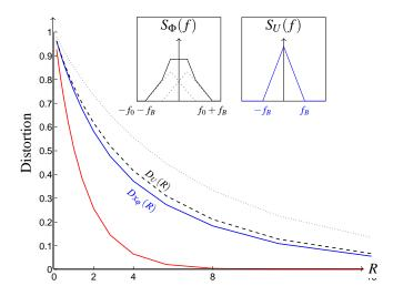
Fig. 7: The DRF of the processes  $X_{\varphi}(\cdot)$  of (45) (blue), the DRF of the baseband process  $U(\cdot)$  (dashed), and the lower bound of Proposition 3. The PSD  $S_U(f)$  is taken to be the pulse given in the small frame. Proposition 6 implies that  $D_U(R)$  and  $D_{X_{\varphi}}(R)$  coincides for  $f_s > 2f_B$ . Also shown is the DRF of the Gaussian stationary process with PSD  $S_{\Phi}(f)$  (dotted), which gives an upper bound to  $D_{X_{\varphi}}(R)$ .
