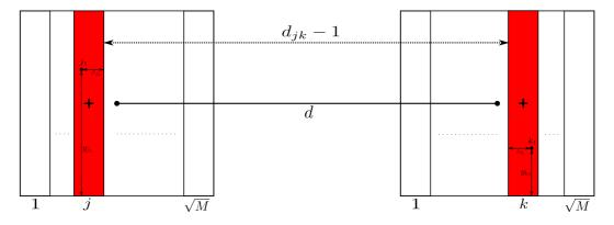
Fig. 4. Two square clusters that have a center-to-center distance d, with each cluster decomposed into  $\sqrt{M}$  vertical  $\sqrt{M} \times 1$  rectangles.  $d_{jk}$  is distance between the centers (marked with cross) of the two rectangles j and k. Moreover, we have the points  $j_1(x_{j_1}, y_{j_1})$  and  $k_1(x_{k_1}, y_{k_1})$  in the rectangles j and k, respectively.
