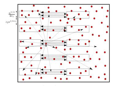
Fig. 1.  $\sqrt{n} \times \sqrt{n}$  network divided into clusters of size  $M = \frac{n^{1/4}}{2c_1} \times \frac{n^{1/2}}{4}$ . Two clusters of size M placed on the same horizontal line and separated by distance  $d = \frac{n^{1/2}}{4}$  pair up and start back-and-forth beamforming. The vertical separation between adjacent cluster pairs is  $c_2 n^{1/4+\epsilon}$ .
