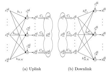
Fig. 1. System model of the uplink and downlink C-RAN.
