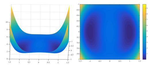
**Figure 2:** Function landscape of (1.1) for x = [1;0] and  $m \to \infty$ . The only local and also global minimizers are  $\pm x$ . There are two saddle points near  $\pm [0; 1/\sqrt{2}]$ , around each there is a negative curvature direction along  $\pm x$ . (Left) The function graph; (Right) The same function visualized as a color image. The measurement vectors  $a_k$ 's are taken as i.i.d. standard real Gaussian in this version.
