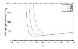
Fig. 7. Average age with respect to codeword length for the M/G/1/1 without preemption scheme with FR-HARQ. We assume the update has 100 information symbols,  $\lambda=1,\,k_s=20$  and  $k_p=100/k_s$ .
