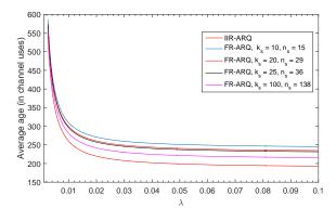
Fig. 6. Comparing the performance of the FR-HARQ for the M/G/1/1 without preemption scheme when varying the number of information symbols in each packet. We assume the update has 100 information symbols,  $\delta = 0.2$ ,  $k_p = 100/k_s$ .  $n_s$  is chosen to minimize the average age.
