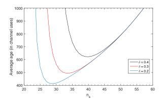
Fig. 5. Average age with respect to codeword length for the M/G/1/1 with preemption scheme with FR-HARQ. We assume the update has 100 information symbols,  $\lambda=0.0066,\,k_s=20$  and  $k_p=100/k_s$ .
