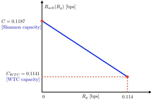
Fig. 4. Achievable rate  $R_{ach}$  as a function of  $R_g$  under the proposed LV-WTC scheme for an  $\mathbf{H}_n$  whose columns are partitioned into  $|\mathcal{G}| = 2^{nR_g}$  exclusive groups with equal cardinality. When  $\mathbf{H}_n$  is full column rank,  $R_g$  increases and  $R_{ach}$  approaches  $C_{WTC}$ , whereas when it is of rank one,  $R_g$  decreases and  $R_{ach}$  approaches  $C$ .
