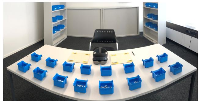
Figure 1: 180° view of the experimental setup. Screws are located on the workpiece carrier, nuts and washers in the picking bins.
