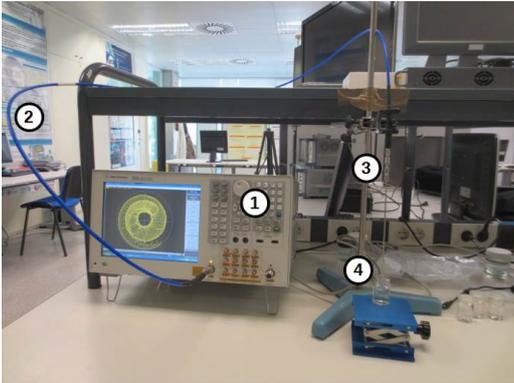
① Vector Network Analyzer (VNA)    ③ Coaxial Probe
