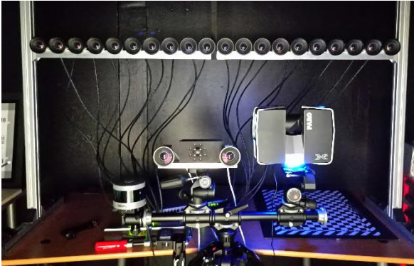
Fig 2. The sensor array used for testing. On the top, 20 identical calibrated Basler cameras. Bottom row: Velodyne VLP-16, Basler ToF, Faro Focus
