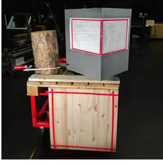
Fig 1. The test scene consisting of a pallet loaded with a small log, a container with a 90° degree angle and a smooth plane. The pallet is set on a wheeled platform to allow changing the distance from the cameras
