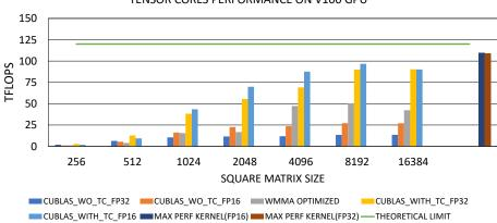
TENSOR CORES PERFORMANCE ON V100 GPU
