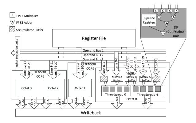
Figure 13: Proposed Tensor Core Microarchitecture
