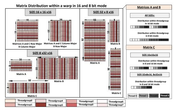
Figure 8: Distribution of operand matrix elements to threads for tensor cores in the RTX 2080 (Turing).
