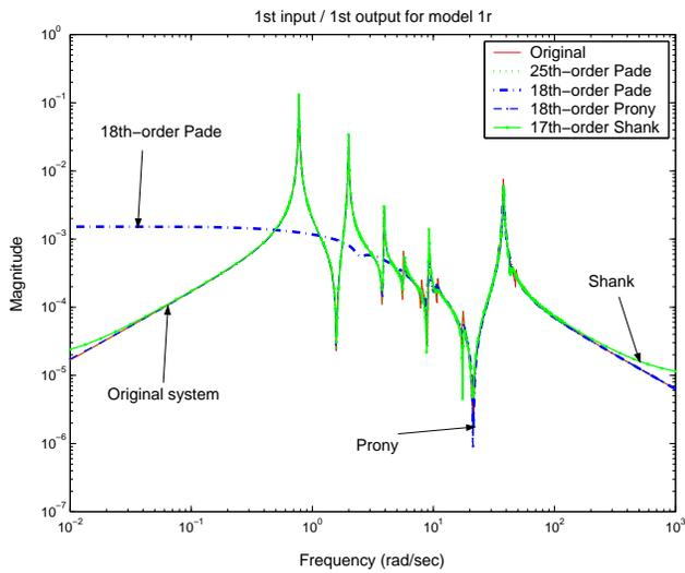
Figure 5. Magnitude response for the international space-station example.
